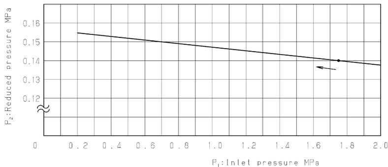
Reduced pressure is set to 0.14 MPa when inlet pressure is 1.75 MPa. The chart indicates a variation in reduced pressure when the inlet pressure is changed from 0.2 to 2.0 MPa.
